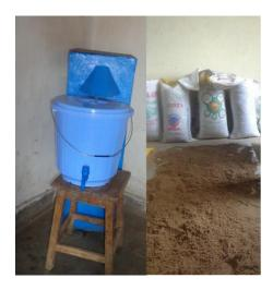
Biosand water is a filter made from concrete with sand and gravel well treated installed inside which helps to make clean the dirty water and removes pathogens, viruses, protozoa, and bacteria.
